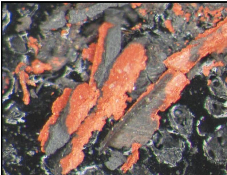
**Sample 22/2** – optical microscopy (magnification 70X). Visually the same two layers of coatings (red base coat and black top coat) as in sample 22/1 were recognized.
